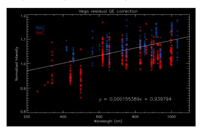
Figure 16: Residual QE correction derived from Vega using the newly-derived correction factors. The fit line is applied to the QE correction function for both cameras, ensuring that the camera-to-camera ratio remains constant with filter.
