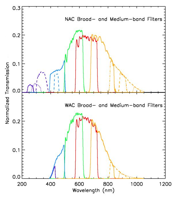
Figure A. 1: Full-system transmission for medium and broadband ISS filters. For the NAC: purple corresponds to UV1 (solid), UV2 (dotted), and UV3 (dashed), blue to BL1 (solid) and BL2 (dashed), green to GRN, red to RED, and orange to IR1 (solid), IR2 (dot-dashed), IR3 (dashed) and IR4 (dotted). For the WAC: purple for VIO, blue for BL1, green for GRN, red for RED, and orange for IR1 (solid), IR2 (dashed) and IR3 (dotted); IR4 and IR5 not shown. From Porco et. al. (2004).
