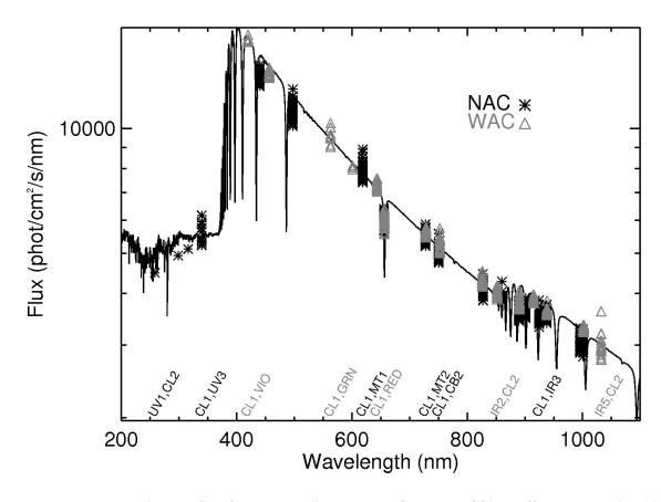
Figure 11:Corrected Vega flux for NAC and WAC as a function of filter effective wavelength. From West et. al. (2010).
