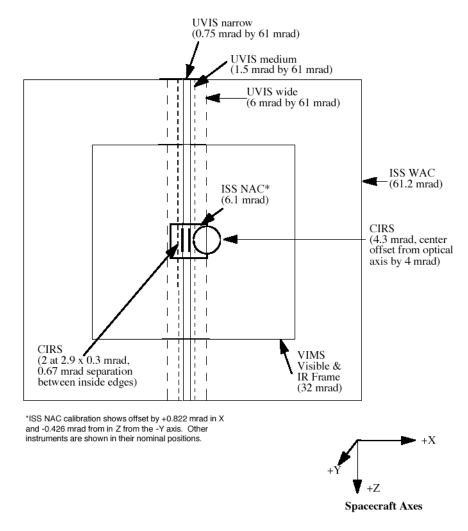
Figure 2: Fields of view of optical remote sensing instruments on Cassini. From Porco et. al. (2004).
