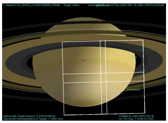
Figure 5: Example of a typical NAC mosaic of Saturn visualized by the Pointing Design Tool (PDT). This particular observation is a 2x2 movie in multiple filters, intended for the study of atmospheric dynamics. From Porco et. al. (2004).
