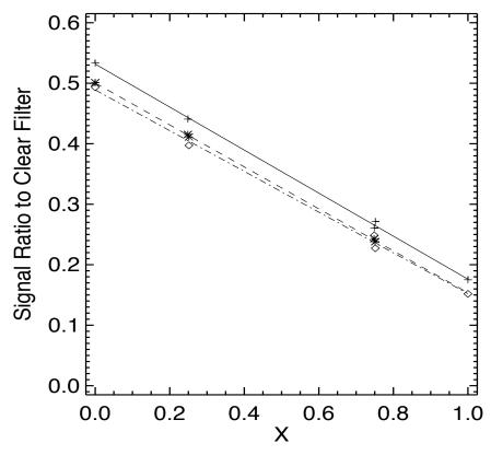
Figure 13: The ratio of the signal in each of three visible polarizers to the signal in the CLR filter (each paired with the BL2 filter) are shown as a function of  $\mathbf{x} = \mathbf{Cos^2}(\boldsymbol{\vartheta})$ . The measurements are shown as symbols for the three polarizers and the straight lines are linear fits to the measurements.
