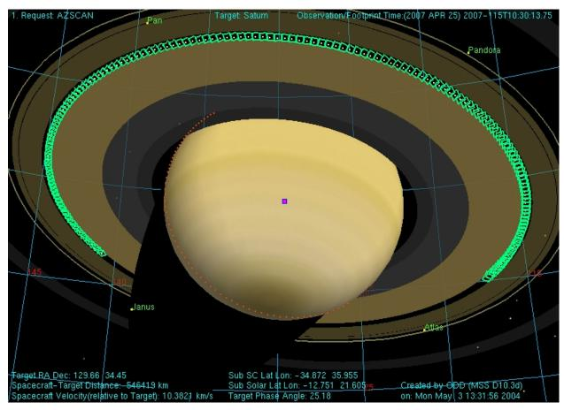
Figure 6: Example of a NAC azimuthal scan (AZSCAN) observation of the outer B-ring edge and Cassini Division at moderte phase and high sub-spacecraft latitude.
