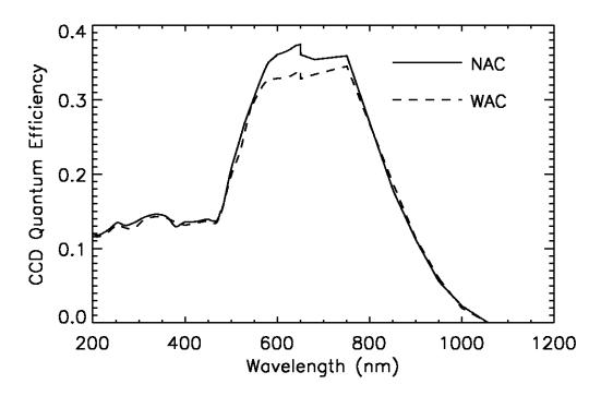
Figure A. 6: ISS CCD quantum efficiency (electrons per incident photon) as a function of wavelength. From Porco et. al. (2004).
