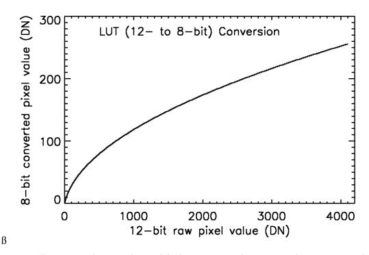
Figure 3: Illustration showing the modified square-root function used to convert 12-bit data to 8 bits in LUT mode. From Porco et. al. (2004).
