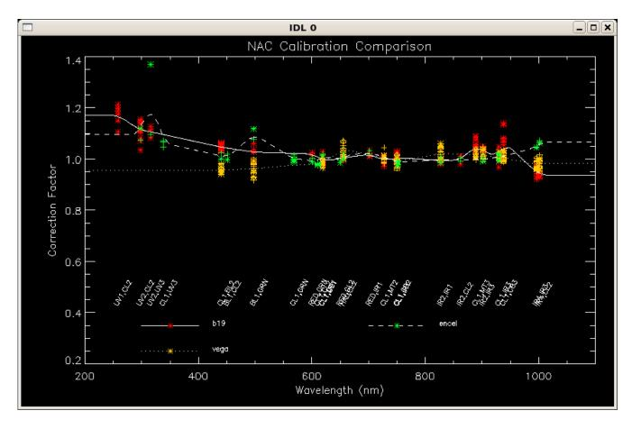
Figure 15: Intermediate NAC correction factors derived from Vega, Enceladus, and the "Bright 19" stars, and normalized to the CL1/GRN value for Vega. Lines have been drawn through the filter averages for each target.
