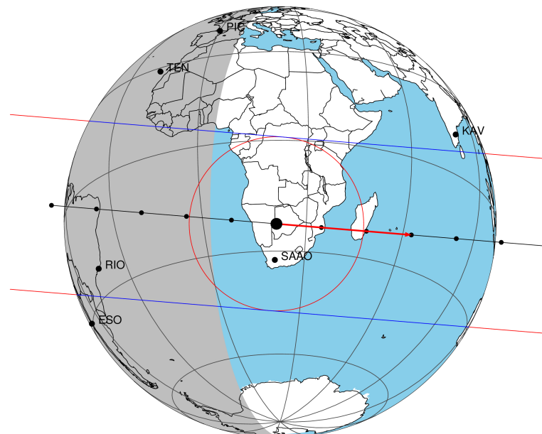
2047-03-05T05:53:05.1700 α: 18 11 52.8783 δ: -22 20 10.393 C/A 0.008" PA 184.11 deg v_sky +22.20 km/s D 10.32 AU Credit: Styled after SORA/Lucky Star
